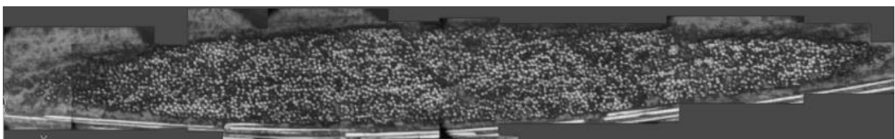
Fig. 3. Cross-section of carbon fibers in a thread
